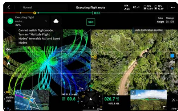
Tahi New Zealand - Drone Flight Dashboard - LiDAR Forest Mapping Photo credit: @Tahi
